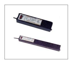
The office range of filtered protected outlets provide surge and transient suppression for computer and office related equipment resulting from mains bourne noise and induced lightning. Available in different plug standards and variations in number of sockets, these units have an integral. EMI/RFI filter, heavy duty surge arrestor, thermal circuit breaker and fault indicator. Failsafe protection is provided by the inclusion of Clearline's new "thermo-trip" technology.
