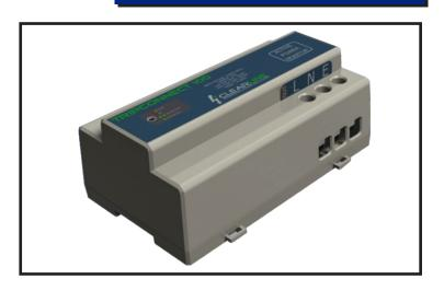
The new 100A Tripoconnect system can be included in domestic and small business distribution boards to eliminate power surges emanating from load shedding. In the case of load shedding, the unit will keep the supply to the installation off until all preset parameters have been complied with and after a short delay, reconnect the supply automatically. The unit will protect against neutral loss and phase failure.
