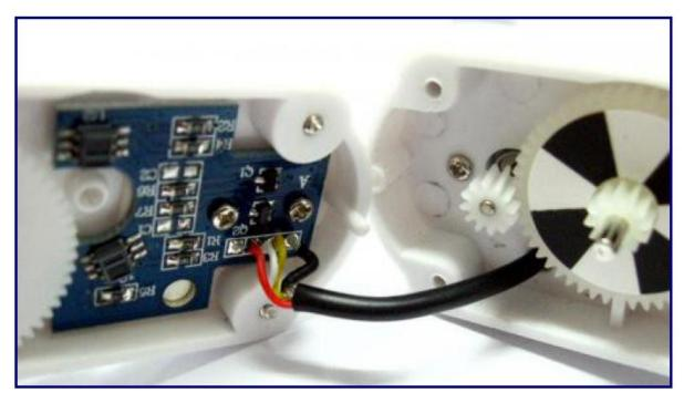
A quadrature encoder, also known as an incremental rotary encoder measures the speed and direction of
