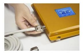
STEP 2 Connect outdoor and indoor antenna with cable.Connect outdoor antenna to "BTS" port in repeater through cable.
