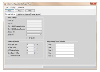
Connect the Falcon to the correct COM port and click on the read button.
