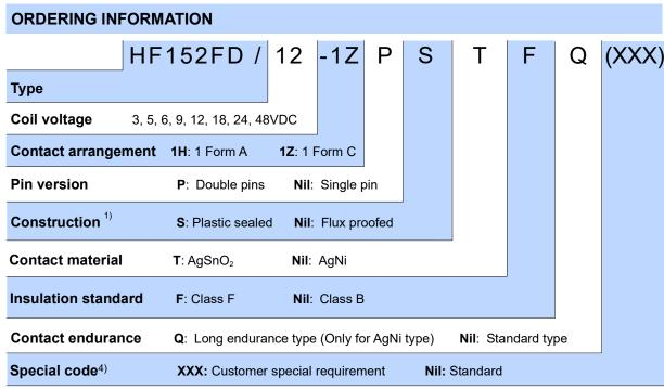
Notes: 1) Under the ambience with dangerous gas like H2S, SO2 or NO2, plastic sealed type is recommended; Please test the relay in real applications.
