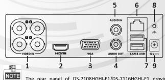
The rear panel of DS-7108HGHI-F1/DS-7116HGHI-F1 provides
