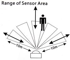
Detection angle: 120° Face sensor straight forward occasions Sensor sensitivity: Low to 4M (Mounting height: 2.5M)
