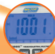
6000 Count LCD display with 61 segmented bargraph
