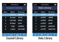
Press the ▲ or ▼ button to select the corresponding cable name. Press the → button once to enter the corresponding cable measurement. Press the → button once to enter the current cable details.
