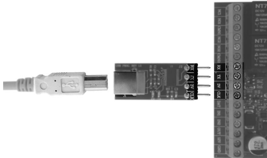
Fig. 3.3 – USB Programmer board connection
