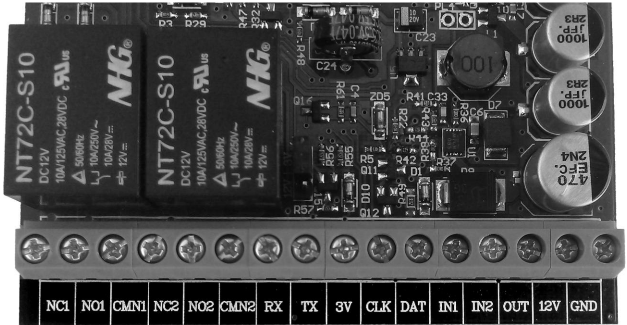
Fig. 3.1 – GSM Communicator connection terminals
