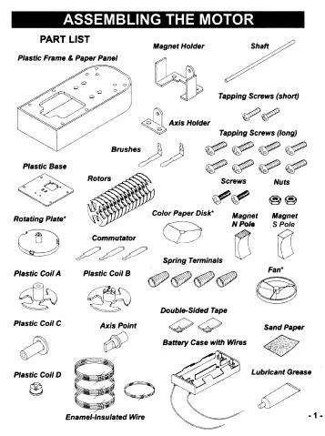
Note: parts marked with an asterisk are not required for assembly, but are used during experiments.
