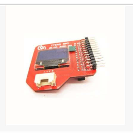
There are seldom OLED add-ons customized for Raspberry Pi in the open source hardware market. In a lot of projects, we only need to display little information such as the state of system or IP. What's more, when we have a high requirement for its portability, it's unsuitable to connect a big screen to Raspberry Pi via HDMI interface. Thus, a tiny OLED add-on can satisfy this demand.
