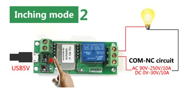
The second wiring way is to connect NC and COM with an appliance. In this way, when users press the setting button or use the APP to turn off, connected appliance will be turned off for 1s and then auto turned on.
