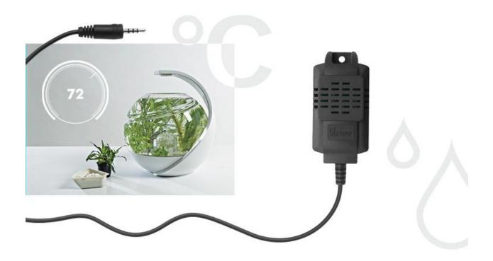
Precision Relative Humidity Sensor ± 3% RH (max), 0-80% RH High Accuracy Temperature Sensor ± 0.4°C (max), -10 to 85°C 0 to 100% RH operating range Up to-40 to +85°C operating range Wide operating voltage (2.2 to 3.6 V) Low Power Consumption Factory-calibrated, digital output Excellent long term stability
