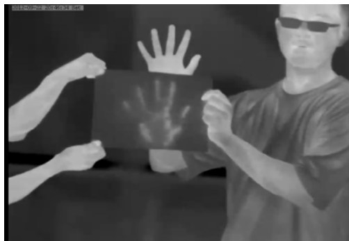
Residual heat detection
