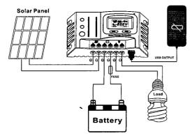
As figure, first connected the battery to controller correct poles. In order to avoid short circuit, please screw the cable of battery to the controller in advance, then connected to battery poles secondly. If your connection is correct, the LCD displaying will show battery voltage and other technical data. If LCD no displaying, please check the fault. The length of cable between battery and controller as shorter as possible. Suggest to 30CM -100CM.
