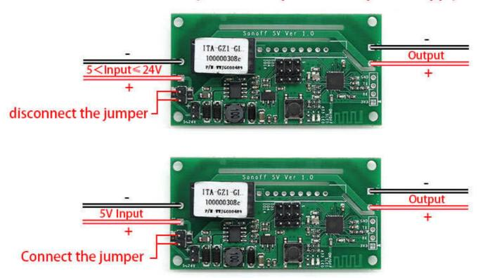
Isolated Mode: WIFI circuit and relay circuit can be isolated
