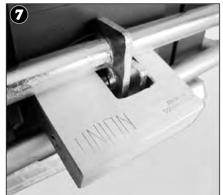
7 With the front bar fully engaged with the overstrap, secure the assembly by locking a good quality padlock through the aligned barrel holes on the overstrap and front bar.
