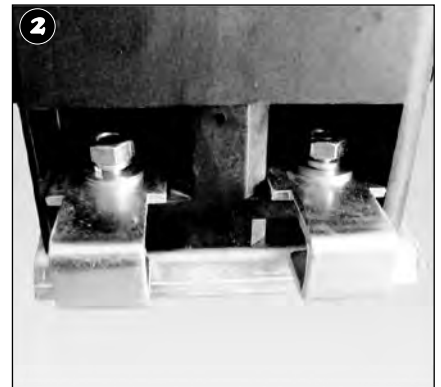
2 Re-fasten the washers and nuts to the retaining studs to secure the brackets.
