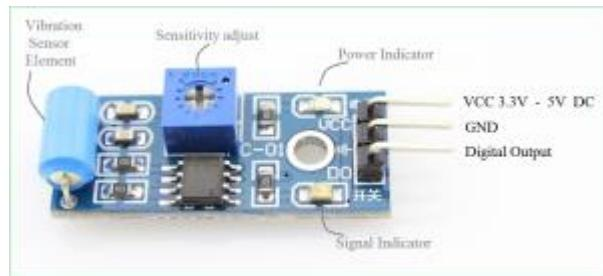
This sensor module produce logic states depends on vibration and external force applied on it. When there is no vibration this module gives logic LOW output. When it feels vibration then output of this module goes to logic HIGH. The working bias of this circuit is between 3.3V to 5V DC.
