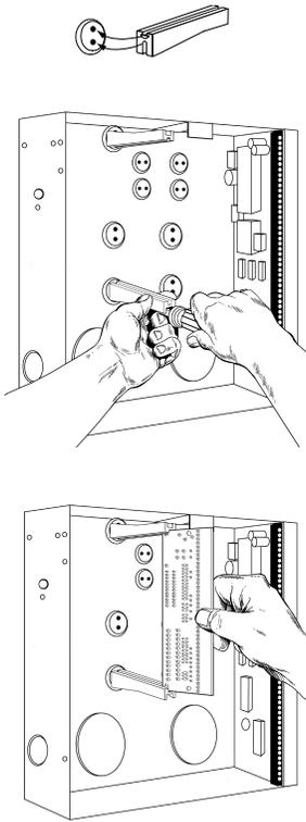
Inside the can, several 2-holed insertion points have been constructed. This allows for either vertical or horizontal placement of the modules. Notice that each insertion point has two sizes of holes – a larger hole and a smaller hole.
