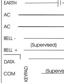
KEYPAD POS AND AUX + TERMINALS ARE LIMITED TO 1 AMP.
