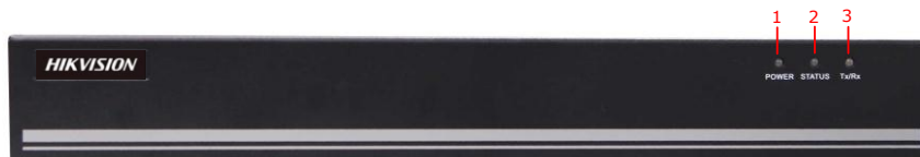
Figure 2.3 Front Panel of DS-6708 and DS-6701/6704/6708-SATA
