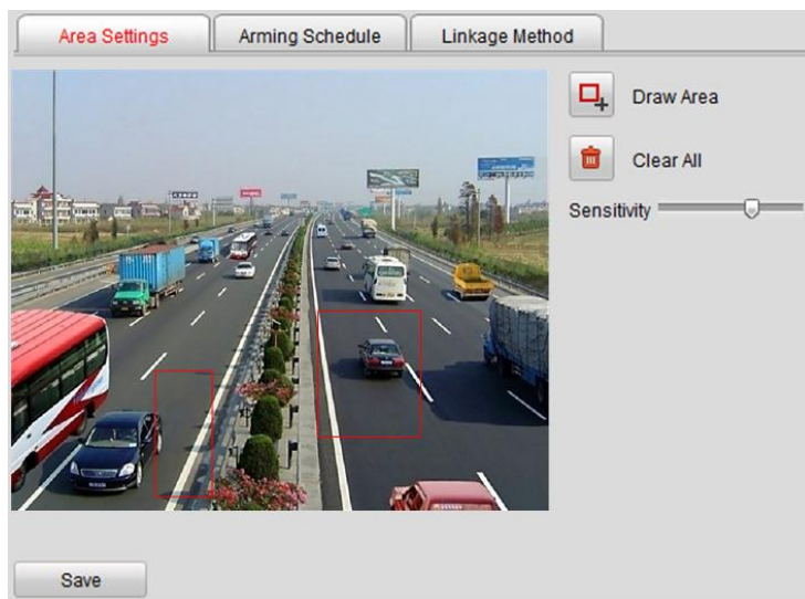
Figure 8.11 Motion Detection-Area Settings
