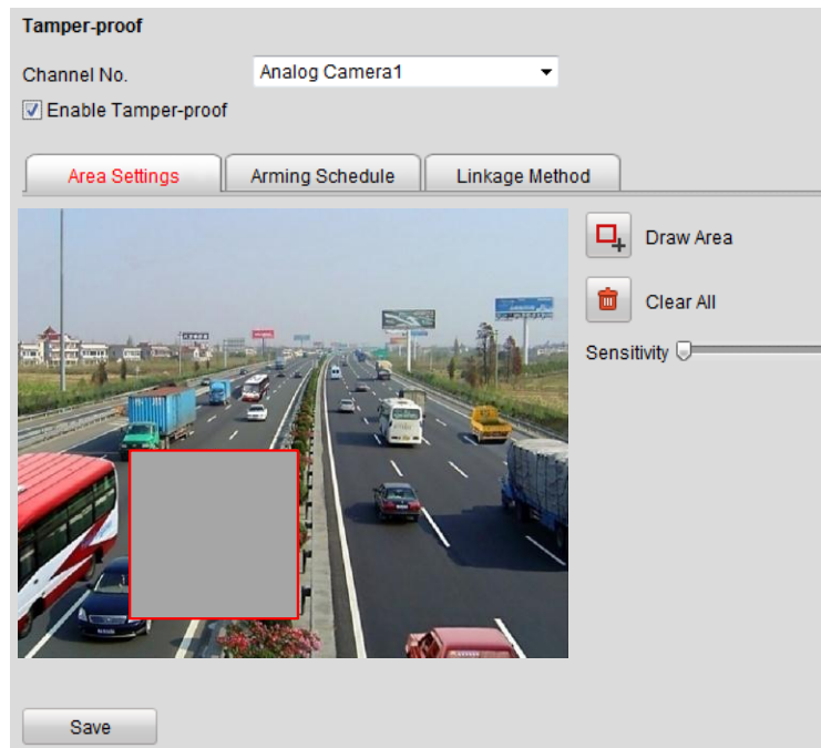
Figure 8.22 Tamper-proof Alarm Settings
