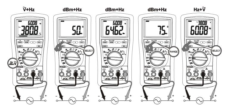
Note: Hz Input sensitivity varies automatically with voltage (current function alike) range selected. 1V range has the highest and the 1000V range has the lowest. Auto-ranging measurements normally set the most appropriate trigger level. You can also press the **RANGE** button momentarily to select another trigger level (voltage range) manually. If the Hz reading becomes unstable, select higher voltage range to avoid electrical noise. If the reading shows zero, select lower voltage range.
