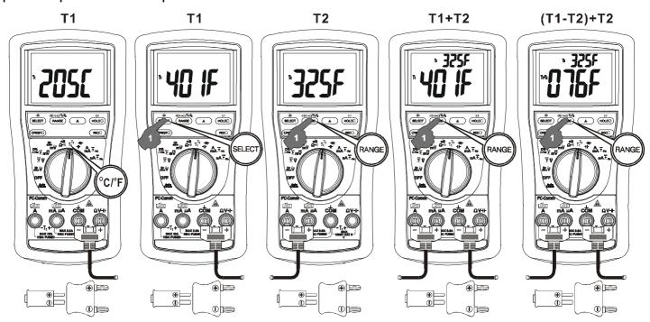
Note: Be sure to insert the banana plug type-K temperature bead probe Bkp60 with correct **+ -** polarities. You can also use a plug adapter Bkb32 (Optional purchase) with banana pins to type-K socket to adapt other standard type-K mini plug temperature probes.
