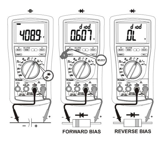
Normal forward voltage drop (forward biased) for a good silicon diode is between 0.400V to 0.900V. A reading higher than that indicates a leaky diode (defective). A zero reading indicates a shorted diode (defective). An OL indicates an open diode (defective). Reverse the test leads connections (reverse biased) across the diode. The digital display shows OL if the diode is good. Any other readings indicate the diode is resistive or shorted (defective).
