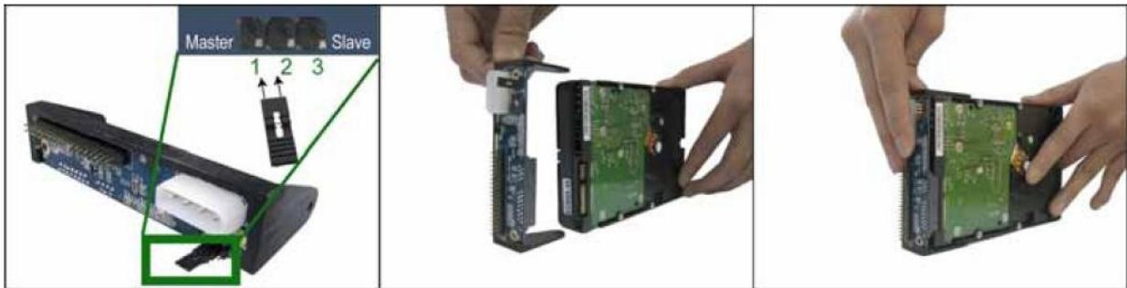
**Step 1.** Insert the jumper into the SATA converter to **set the Master / Slave mode** of the SATA HDD.
