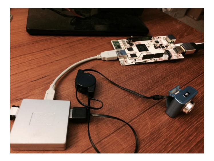
Finally, we see that USB camera is working in scratch for pcDuino:
