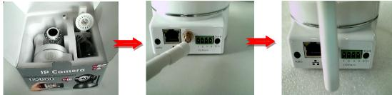
•1.2 Fix the ip camera, insert one end of the network cable to the camera tail Ethernet card interface, on the other end of the RJ45 network interface connected to a router or switch..
