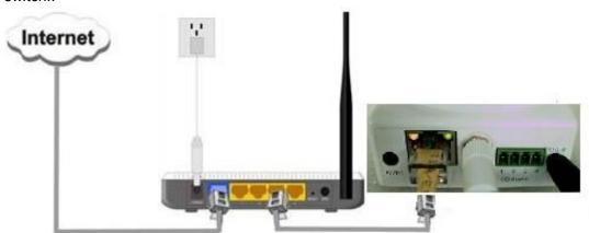
•1.3 The software of IP Camera support windows XP/Vista/windows7 etc. operation system, Pls use the power adapter to connect the DC5V port on the back of the ip camera. Plug the other end to an electrical outlet. Check the card's power indicator light (yellow) and the network indicator (green) is working properly, the camera pan and tilt rotate automatically..
