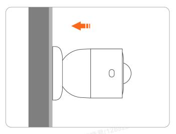
2. Attached to the metal surface with the magnetic base
