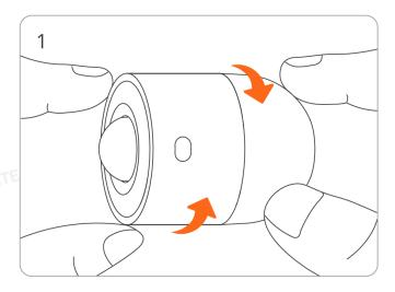
Rotate to open the sensor
