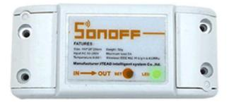
3. Green led quickly blinks one time and repeat, which means device fail to connect to router. In this case, please confirm your Wifi name and password is correct and repair again.
