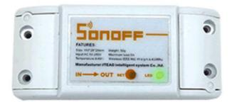
4. Green led slowly blink means device has connected to router and server, but fail to be added in device list. Then try to add the device again.
