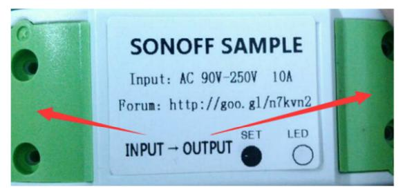
The two terminal connector ports at "INPUT" can connect to input cable L and N randomly, and the two terminal
