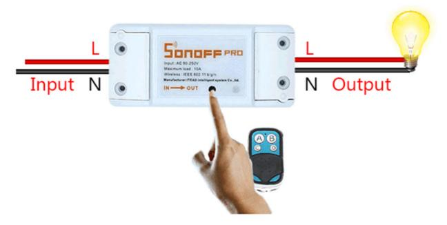
If the Sonoff and Slampher you buy has 433Mhz RF receiver inside, then you can pair them with the <u>RF Remote controller</u>. Quickly press "SET" button on Sonoff and Slampher twice, the red LED on Sonoff/Slampher will flash one time, then press one of the ABCD buttons on the controller once for a few seconds to pair with. If you pair it with A, then you can press A to turn on/off your device.
