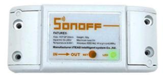
5. Green led quickly blinks twice and repeats, this means the device has connected to router but fail to connect to server. Then please confirm your wifi router works normally.
