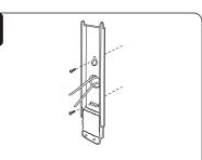
Lead cable in through wiring hole and install bracket on wall upright with fastening screws(2 positions), make sure installtion height is between 0.8-1.2m.
