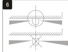
For proper trigger, please don't install detector too farw away from wall surface
