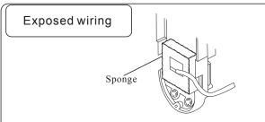
Lead cable in throught detector base and connect to termimals. And lead it out from the lower side of detector base, make sure that cable is between sponge and metal bracket for purpose of water proof, dust proof and anti insects.
