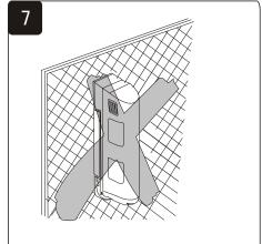
Don't install detector on instable base such as fence and trees
