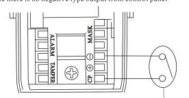
Optional switch O In case there is negative type output or relay output from control panel
