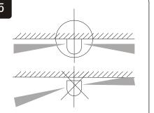
Make correct installation and make sure that detection range is paralle to wall surface
