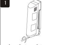
Loose front cover fasten screw and remove front cover. Don't touch lens surface
