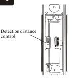
Operator can get needed detection disance by control of 3-grade switch, among which "FAR" grade means 8-12m; "MID" is 4-8m while "SHORT" is 2-4m.
