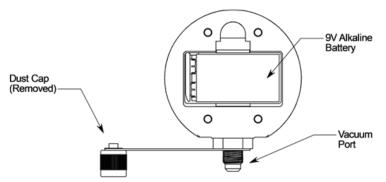
**Rear View (Battery Cover Removed)**
