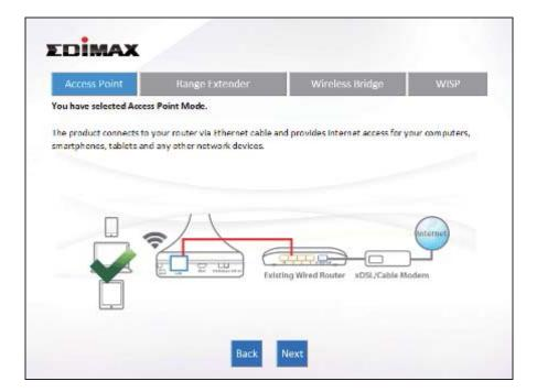
**2.** Connect the network port of your BR-6288ACL to the LAN port of your existing router using an Ethernet cable, then click "Next".
