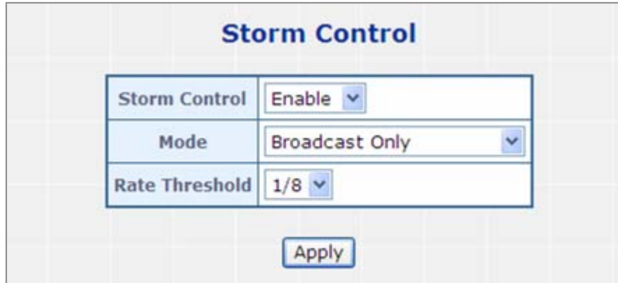
Figure 4-41- Strom Control screen
