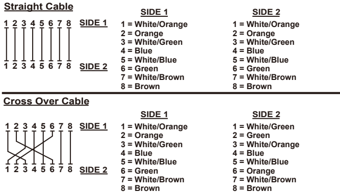
Figure A-1: Straight-Through and Crossover Cable
